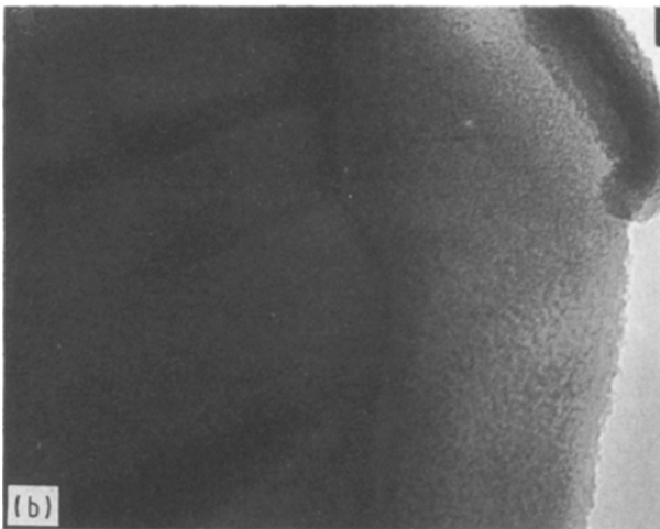
Figure 14 (a, b) TEM morphology of Type I composites containing 40 vol % SiC whiskers after nitridation, showing the nucleation of \alpha -Si 3 N 4 needles.
